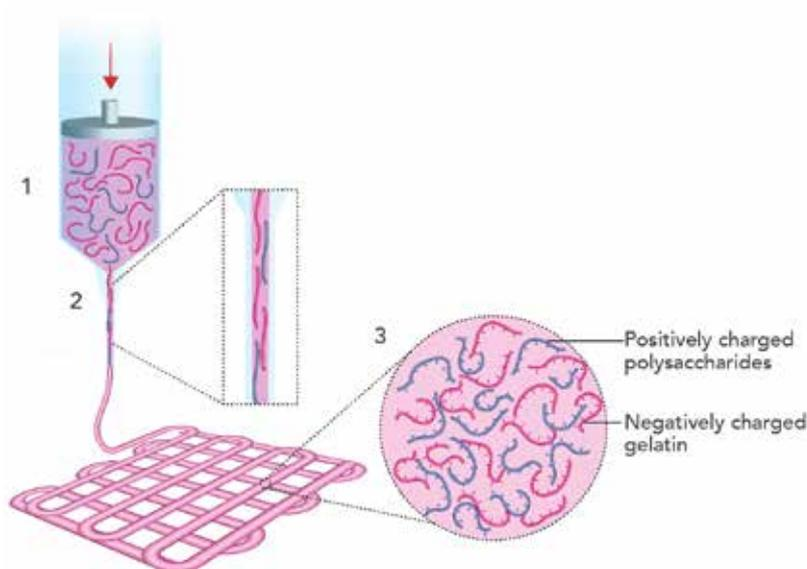
1. In the syringe the gellan chains (blue) form a temporary network with GelMA (red) and induce a gel like viscosity;
